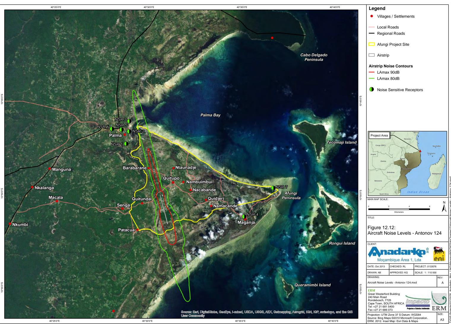
The LAmax 80dB contour for the Cessna 208 falls within the runway area, and hence there is no significant impact from the operation of the Cessna 208.
