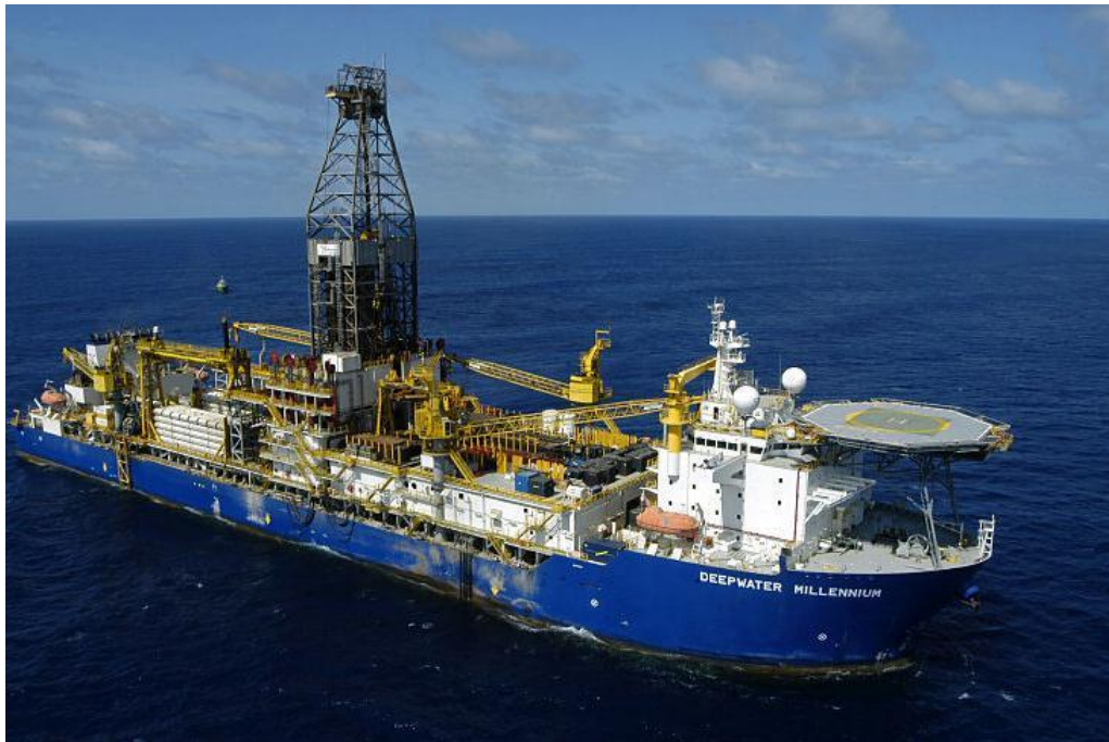
Figure 2.2 – Example of DP Drill Ship
